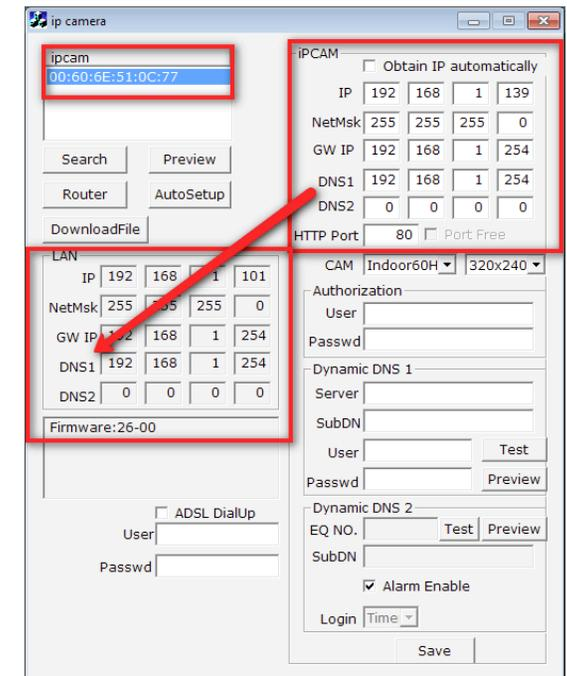
Next select the HTTP port you would like to use to view your camera remotely. The default port is 80. You will now need to open this port within your router to view the camera remotely. If you will only be using this camera on your local network you do not have to open this port on your router.
