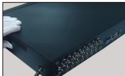
② Loosen the screws on the side to open the cover.
