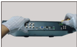
① Loosen the screws on the back.
