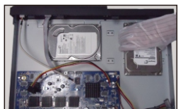
③ Put the HDDs onto the bottom of the machine.
